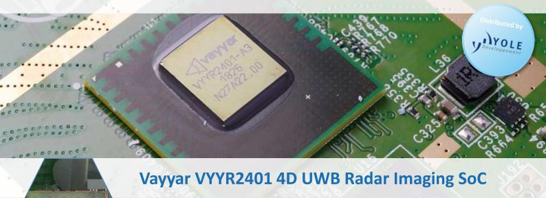
Deep dive analysis of Vayyar's 4D UWB Radar Imaging System-on-Chip from the Walabot Home Fall Detection System.
